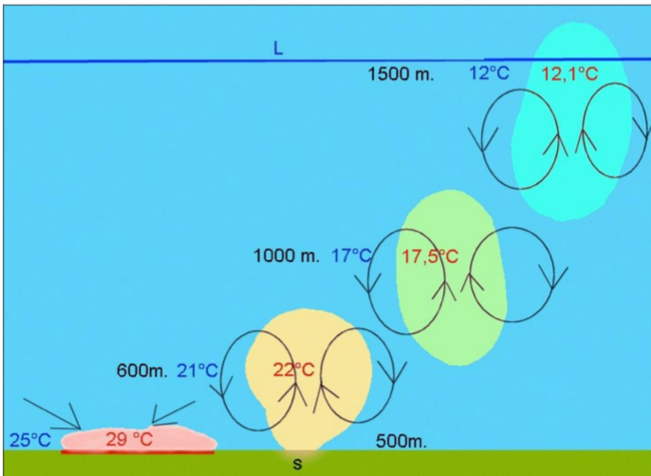
Figure M09: Evolution of the temperature of the air in a rising thermal bubble.
