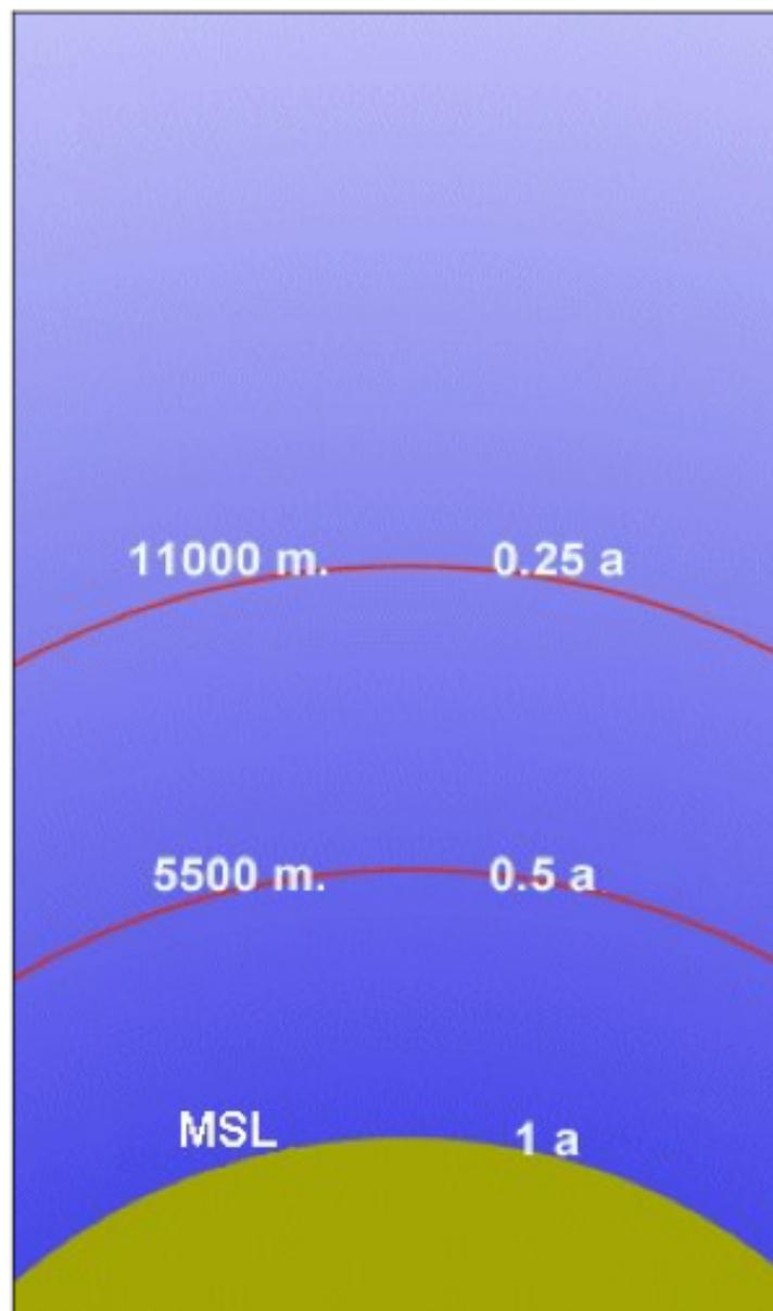
Figure M02: decrease in atmospheric pressure with altitude. Major reference points.
