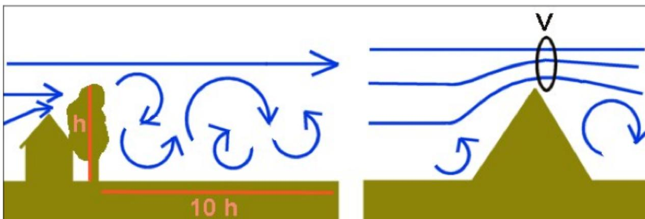
Figure M25: mechanical turbulence
